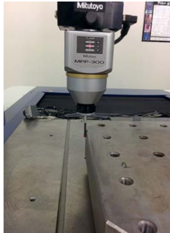
Fig. 10. Mitutoyo MPP-300 scanning probe to measure a 15 mm by 15 mm spatial grid on the CMM
