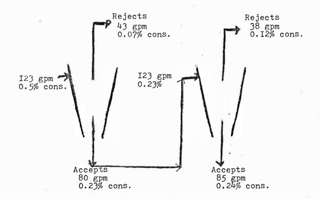
Samples will be taken from the accepts and rejects after each stage. These samples will then be classified on the Clark Classifier and handsheets will be made with the Noble and Wood Handsheet apparatus. (Sample size will be 5 gallons.)
