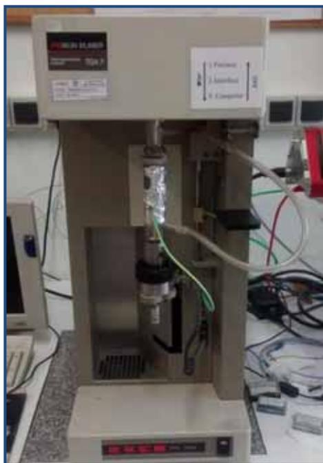
Figura 6.14 Termobalanza TGA (Perkin Elmer (TGA 7)).
