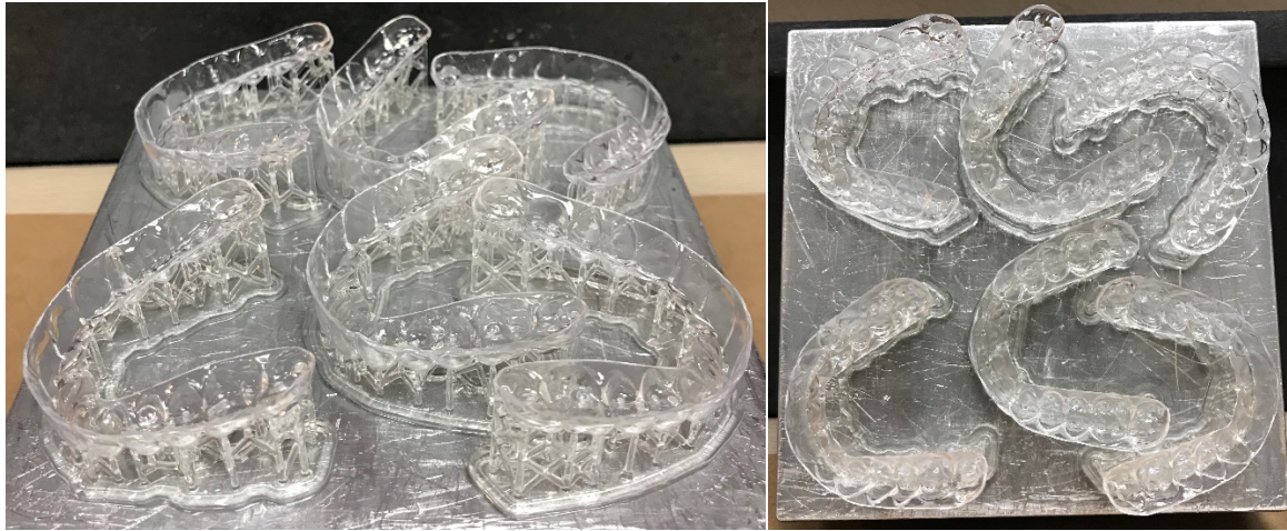
Figure 4. Retainers on the build platform. A total of 6 retainers were printed for each print batch. This is an example of retainers printed at 15 degrees.
