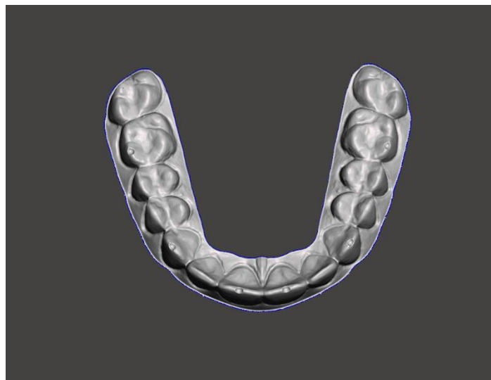
Figure 2. Standard STL file with the reference points on the mesiobuccal cusps of the first molars, the cusp tips of the canines, and the middle of the incisal edges of the central incisors
