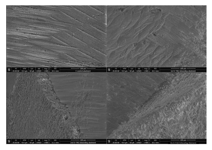
For the crowns, the cameo surface of the control group appeared to be the smoothest. The cameo surfaces of the test samples, G1 Er1, G1 Er2 and G2, appeared to be slightly rougher suggesting the roughness increased from the irradiated glazed feldspathic surface. The intaglio surfaces of all groups appeared to be similar in the roughness. However, the first Er:YAG (G1 Er1) group showed less cement compared to the repeated Er:YAG (G1 Er2) and Er,Cr:YSGG (G2) groups (**Fig 3-6**).
