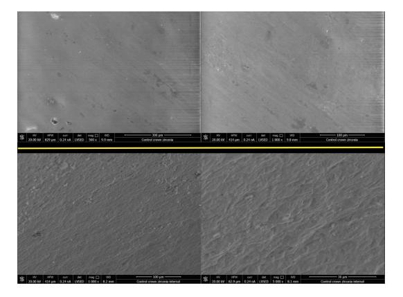
**Figure 4: SEM analyses of Er:YAG lasered zirconia crown after first cementation (G1 Er1)** (Top) Cameo surface of the first time Er:YAG lasered zirconia crown demonstrated slightly rougher than the control. (Bottom) Intaglio surface of first time Er:YAG lasered zirconia crown demonstrated zirconia surfaces similar to the control little cement remaining.
