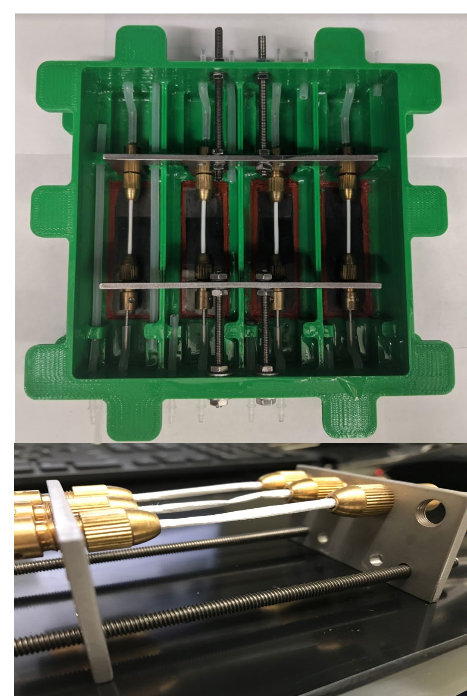
Figure 6. Final assembly of the ETVG chambers. Notice the brackets hold all four of the grafts in place. The actuator will provide motion for all four grafts via the one bracket.
