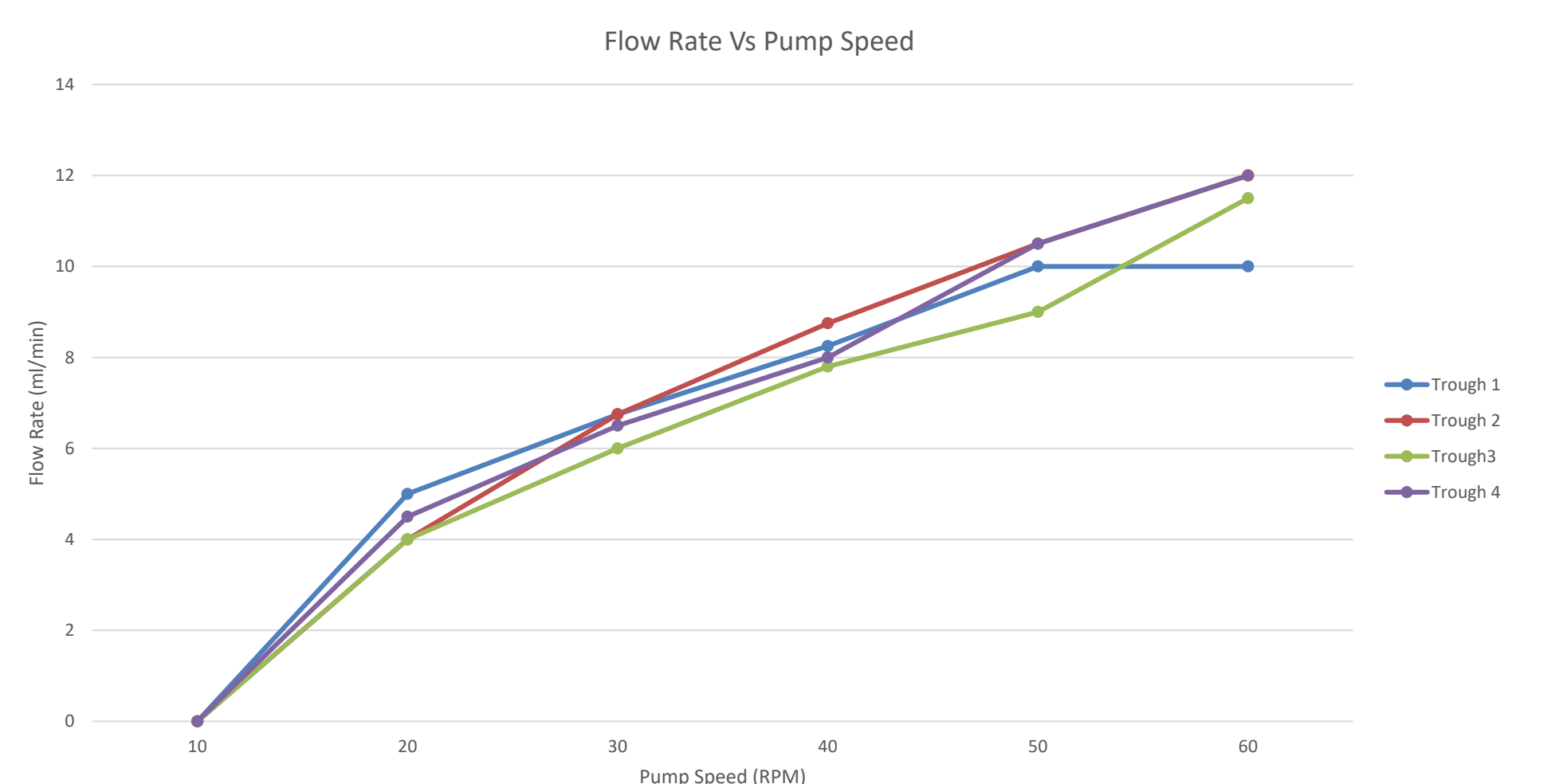
Figure 7. Flow rate from each trough by pump speed. The pump provides a linear increase in flow rate as the speed of the pump increases up to ~40 RPMs. After that, the flow rates vary in a seemingly uncontrollable manner.
