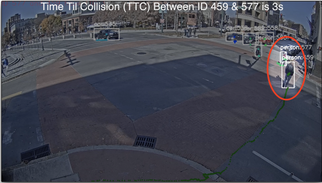
Figure 5.4 A near-miss event being detected between two pedestrians at the intersection of MLK and Georgia Ave., portraying the success of the near-miss approach introduced in this chapter.
