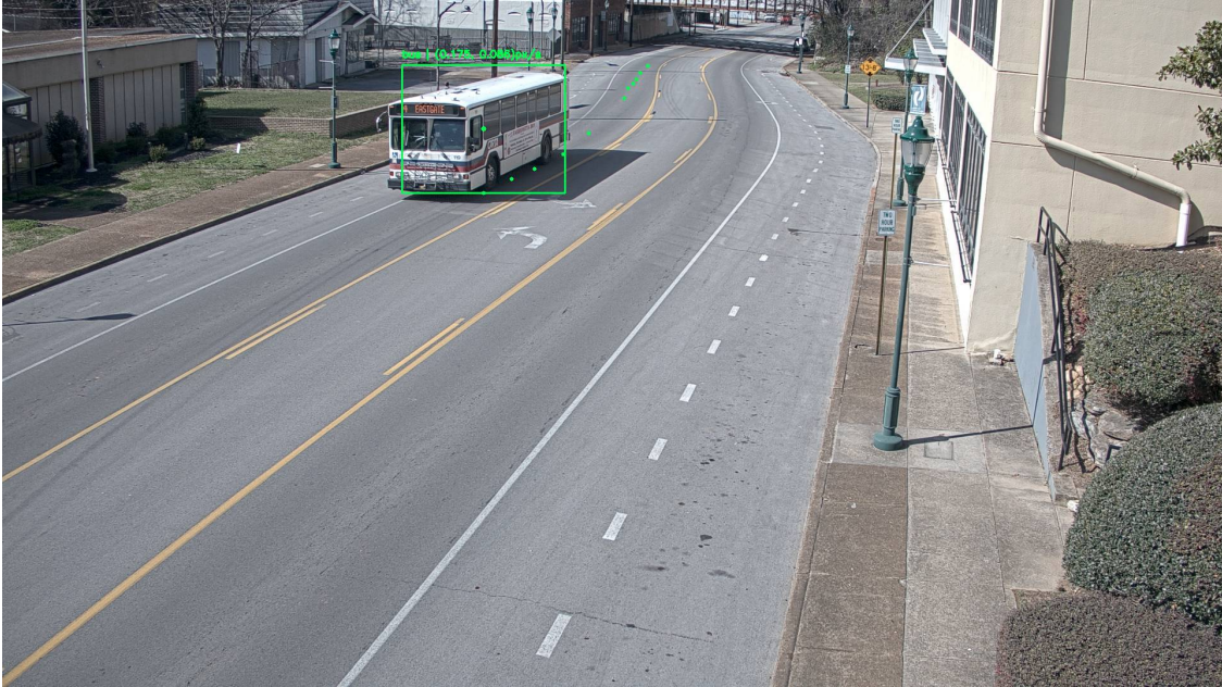
Figure 5.1 Pixel-Relative Velocity drawn above a tracked bus (indicated by the green rectangle) on the testbed. Velocity is being calculated using the data from object tracking, using the delta in time and position for calculation.
