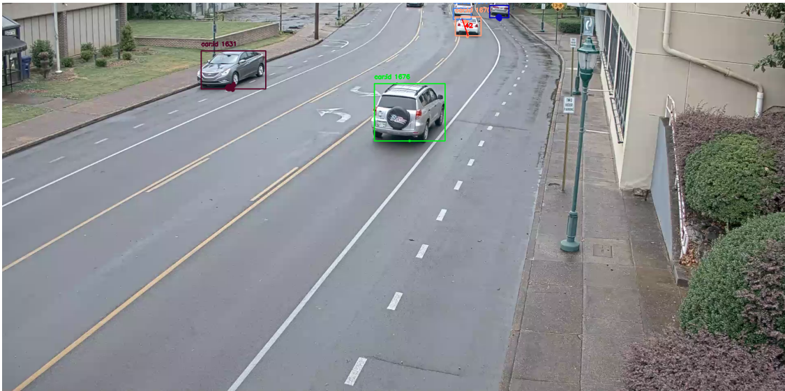
Figure 5.3 A near-miss event being detected between two vehicles at MLK and Peeples St., shown by the red line and number drawn near the top of the image.
