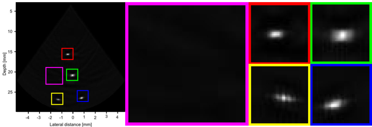
Figure 5.8: A closer look at the EG-CRC reconstruction of the real phantom. Better noise suppression was achieved, and the bottom right wire was reconstructed without the artifact seen in B-CRC (closer look in figure 5.9). 40 dB is the dynamic range.
