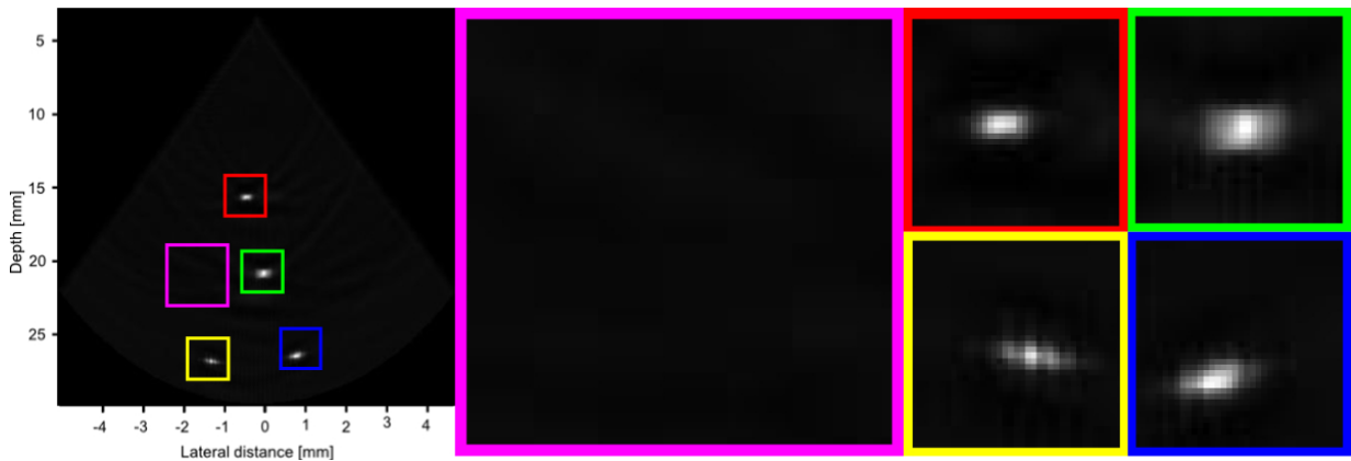
Figure 6.6: A closer look at the EG-CRC reconstruction of the real phantom. Better noise suppression was achieved, and the bottom right wire was reconstructed without the artifact seen in B-CRC (closer look in figure 6.7). 40 dB is the dynamic range.
