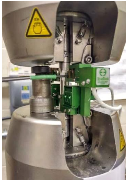
Figure 18. Bi-axial test setup, showing the frame and bi-axial extensometer
