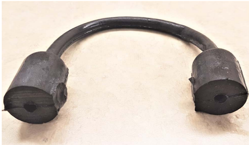
Fig. 3.2. Picture of the PVA-based straight tube vessel before mounting it in the phantom box.
