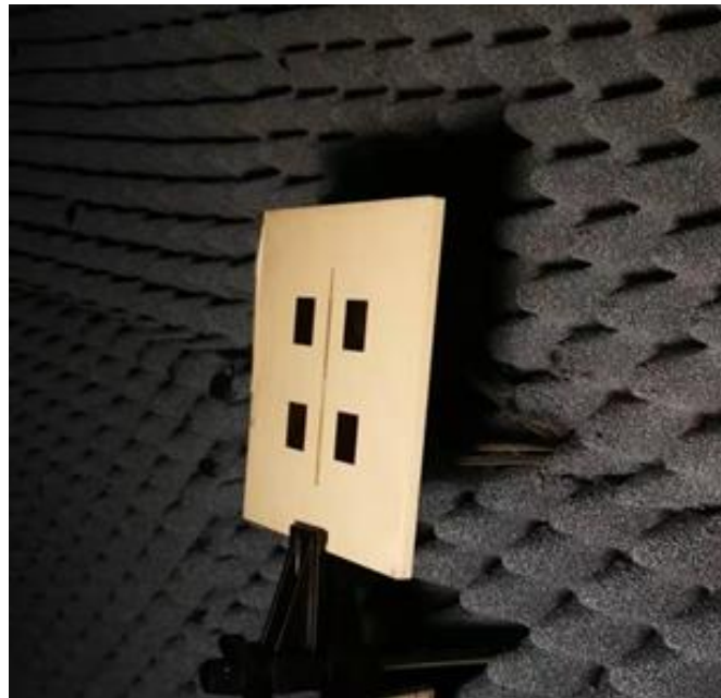
Fig. 3.15 Picture of the antenna array and test environment.
