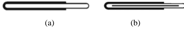
Fig. 3.7 Evolution of the decoupling unit cell [34]. (a) Asymmetric loop resonator with different loop lengths. (b) Wideband loop resonator proposed by [34]
