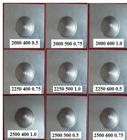
Fig. 4 Components formed as per L9 orthogonal array
