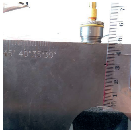
Figure 1: Part of the experimental setup for testing detection algorithm: Krautkramer 2.25 MHz ultrasound transducer on SS 1018 calibration block
