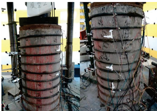
Figure 4 Crack propagation and failure of model 2
