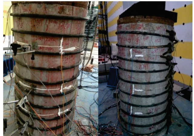
Figure 5 Crack propagation and failure of model 3
