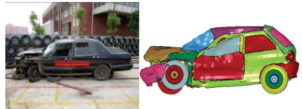
Figure 11 Damage comparison diagram of real sedan and simulation sedan
