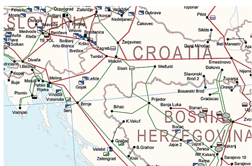
Figure 2 Overview of the Transmission Power System of Croatia and Slovenia (highlighted hydro-power plant Zlatoličje and 400 kV transmission line Melina - Velebit)
