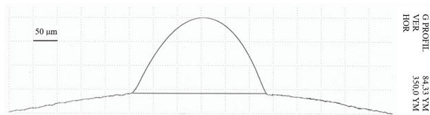
Figure 1 Braille cell G profile measured with Perthometer S8P
