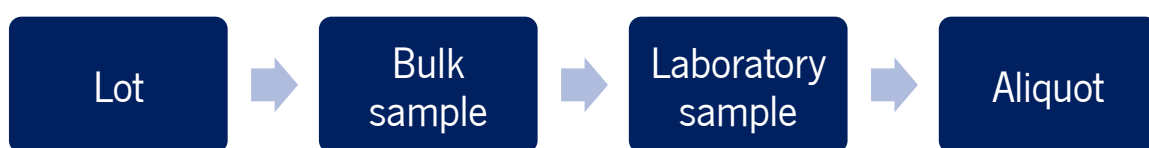
Fig. 1 – Sampling pipeline represented as a flow chart: from lot to aliquot.
