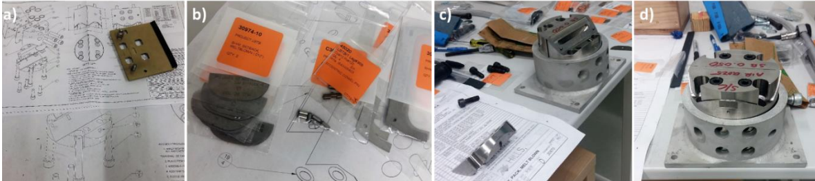
Figure 3. i Die assembly: a) spinnerets plates system, b) small metal parts to define setback and air gap, c) the die incomplete and d) the final state of the die.
