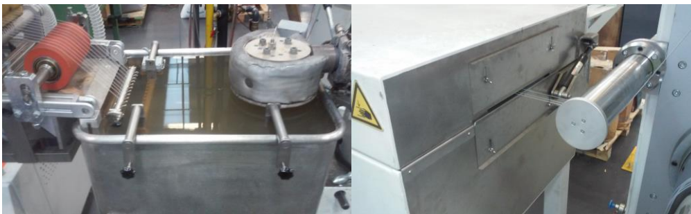
Figure 9 - Company extrusion line. On the left side is presented the vertical extrusion and on the right side the heaters isolation
