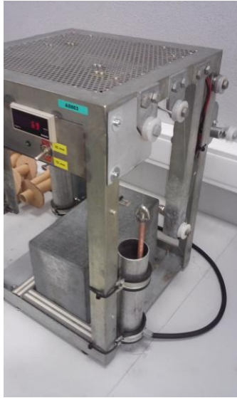
Figure 11 - Abrasion resistance tests installation
