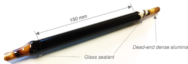
Fig. 1. Image of the resulting composite carbon molecular sieve membrane.
