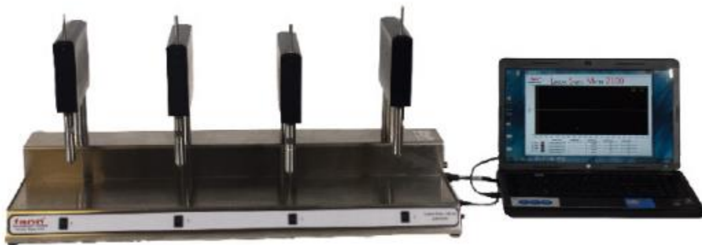
Figure A2: Linear swell meter attached to a data acquisition system
