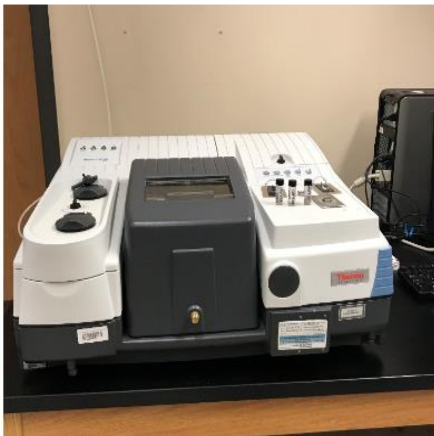
Figure 15- FTIR spectrometer for mineralogy testing
