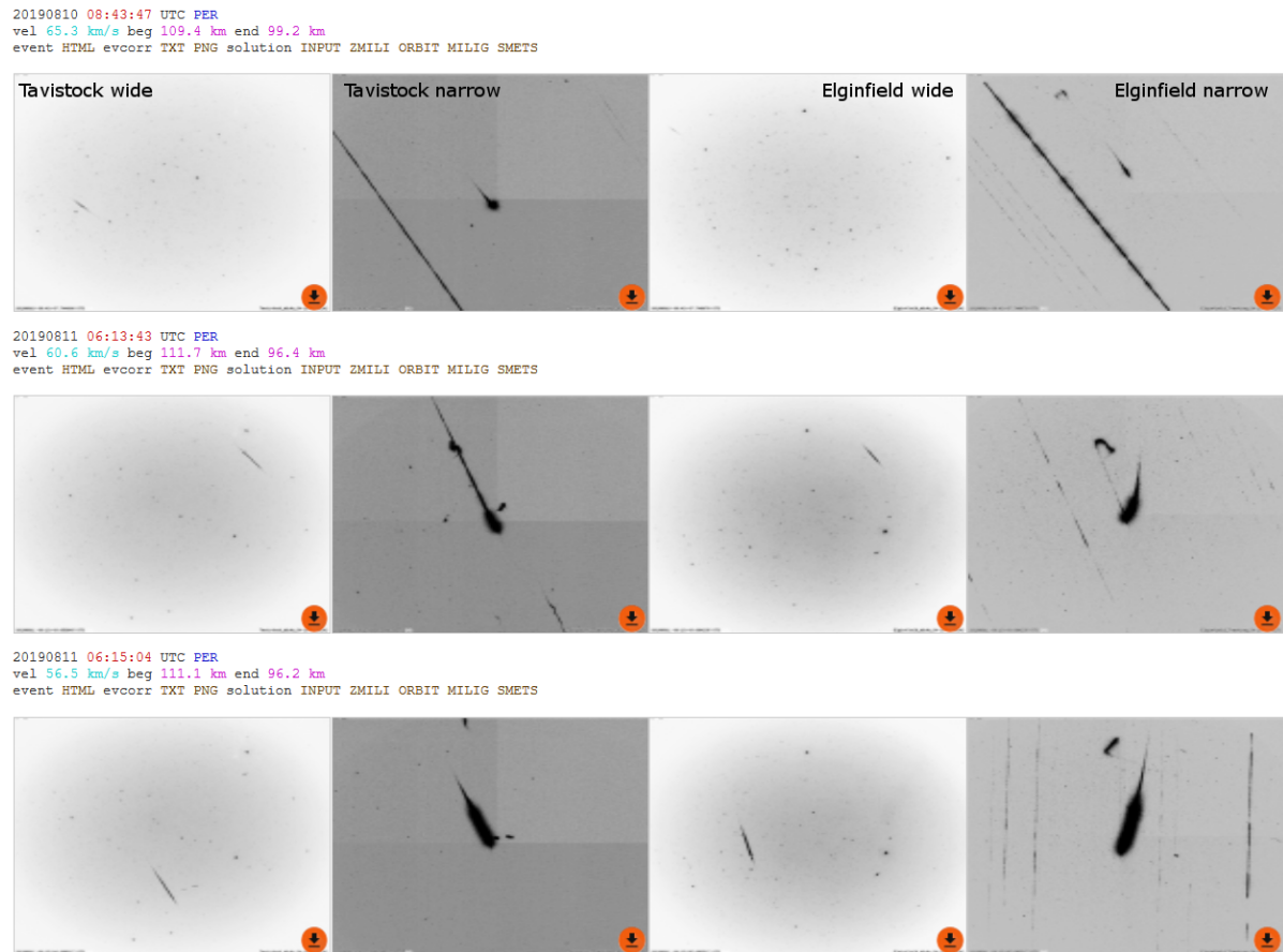
Figure 6.6: Screenshot of the CAMO weblog page showing three Perseids. Co-added video frames from all sites and both wide and narrow field of view cameras are shown.
