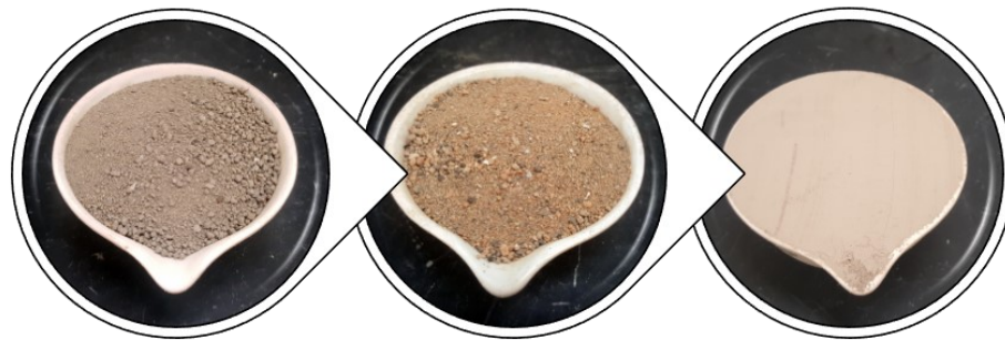
Figure 4-2: Visual aspect from the left to right: raw dried, calcined, ground sediments
