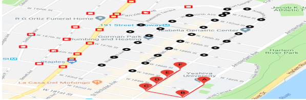
Path A->B->C->D->E->F->Black Zone ->Red Zone The part A->B->C->D->E->F is generated offline. The decision to move from F to Black Zone then to Red Zone is taken online based on available requests. Black Zone – Consists of Black circled nodes. Red Zone – Consists of Red rectangle nodes.
