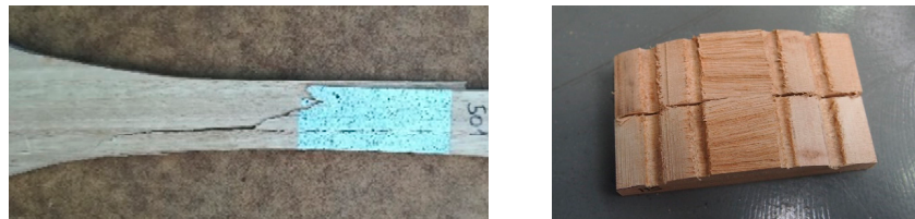
Figure 4. Typical failures in tension parallel to grain (left) and tension perpendicular to grain (right).
