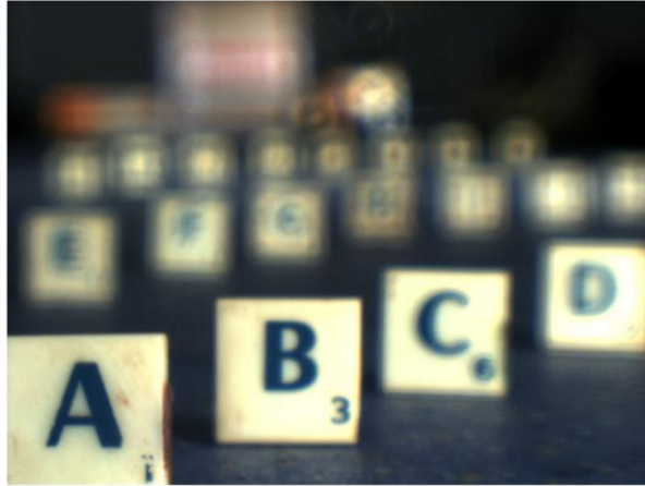
Fig. 13. The 3 D scene imaged by the artificial eye compensated by the monofocal lens ( Media 2 ).
