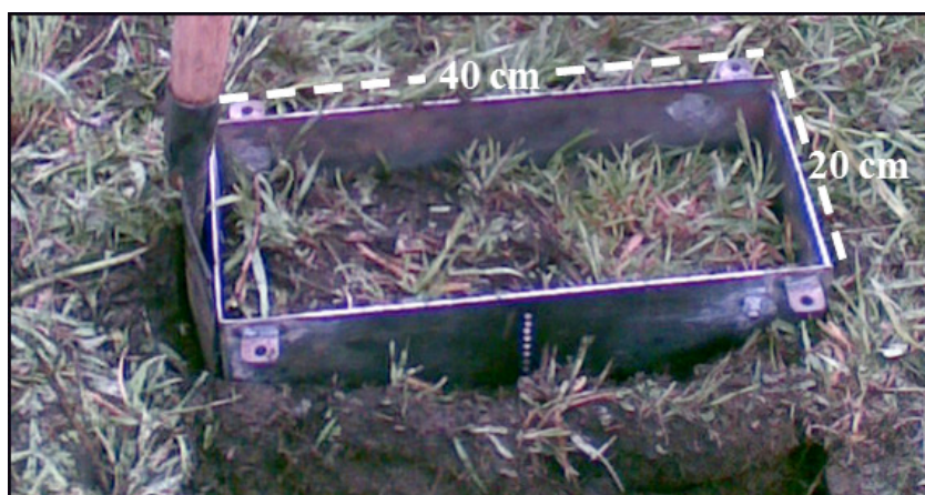
Figure 1. Equipment used for unaltered sample collection on site.
