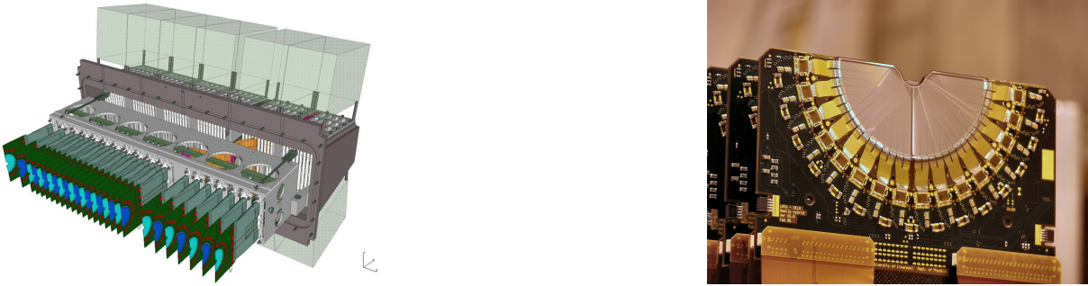
Figure 2.7: Left: a lateral view of the VELO detector. Right: real picture of the VELO sensors.
