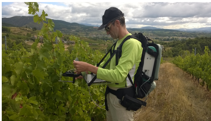
Figure 3: Registering leaf reflectance with a spectroradiometer.
