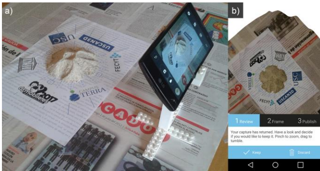
Fig. 1. Scanning real objects with mobile devices and photogrammetry: (a) taking photographs with a mobile device camera and (b) 3D object reconstruction.
