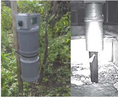
Fig. 1: Mote for snail pest detection based on capacitive sensors (left) and a snail entering the shelter (right).
