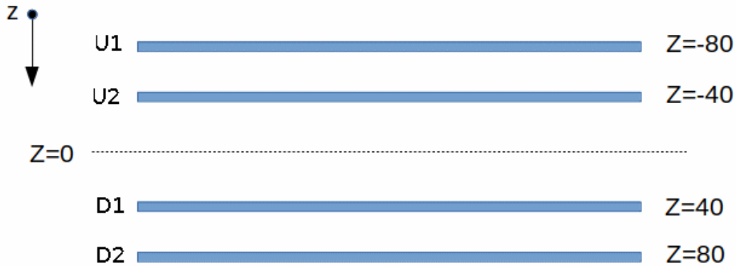
Fig. 5.1 Overview of the physical structure used in the simulations. The target materials will be placed at z = 0 . We took z as positive along the propagation of the cosmic rays. Distances are given in cm.
