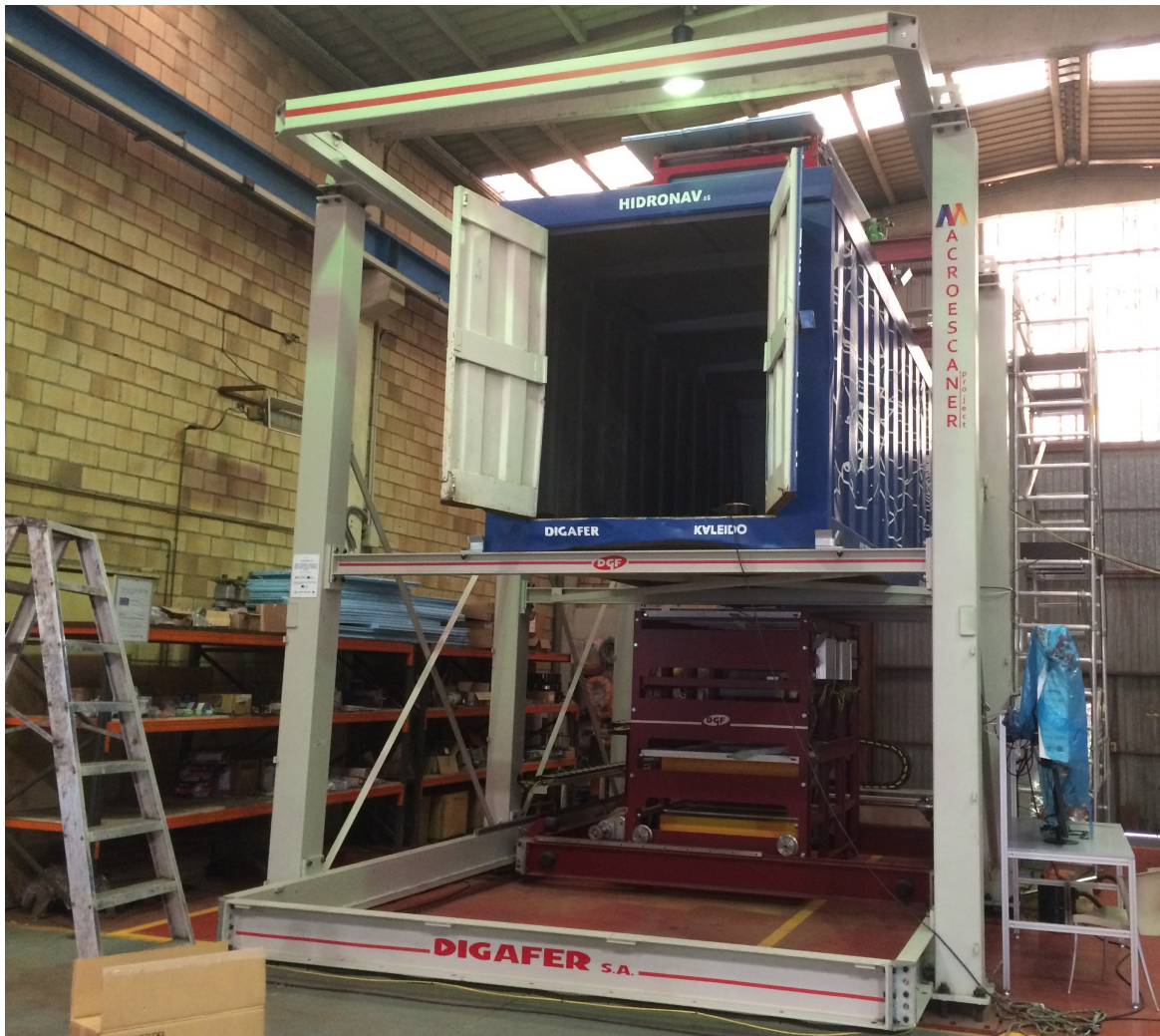
Fig. 8.2 Prototype of the macro scanner structure. Two muTT detectors are placed above the container, and the other two are placed below. The four detectors move at the same time to cover the whole the surface of the container.
