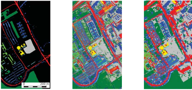
Figure 6. From left to right reference data , and classification maps for SVM and SVM-QS for the Pavia Univ. image.
