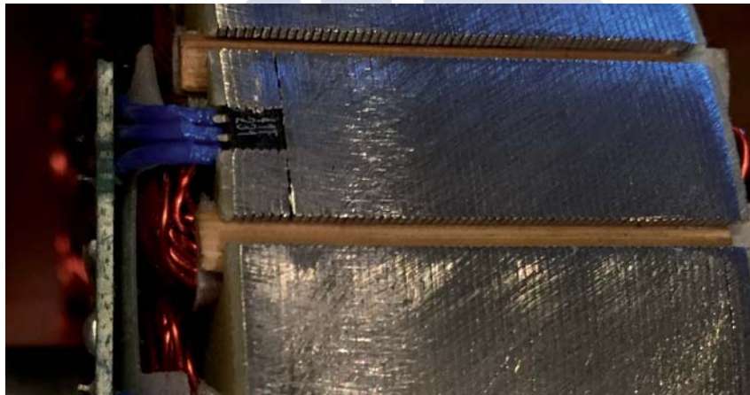
Figure II.4: Lamination detail. Derivative of E-Twow Electric Motor by Kaspars Dambis under license CC-BY-2.0.
