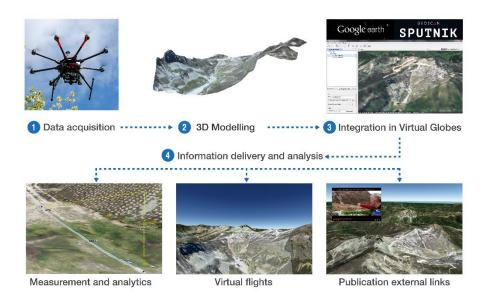
Fig. 1. Workflow for UAV data integration in virtual globes.
