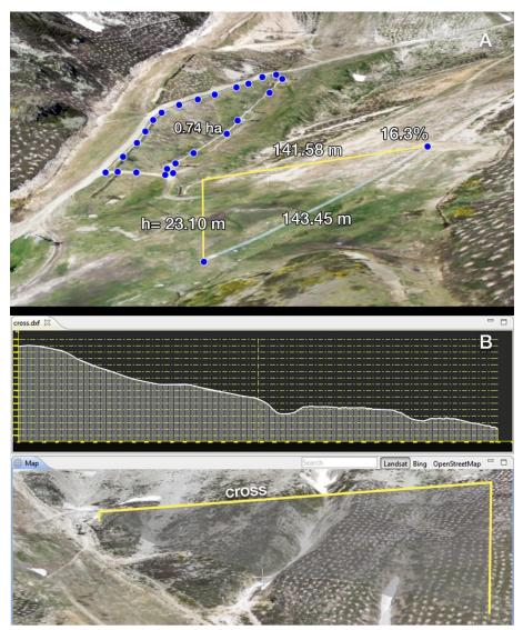
Fig. 4. Measurement tool (a) and cross section tool for profile analysis (b) in Sputnik GIS [image fit: 1.5 columns]
