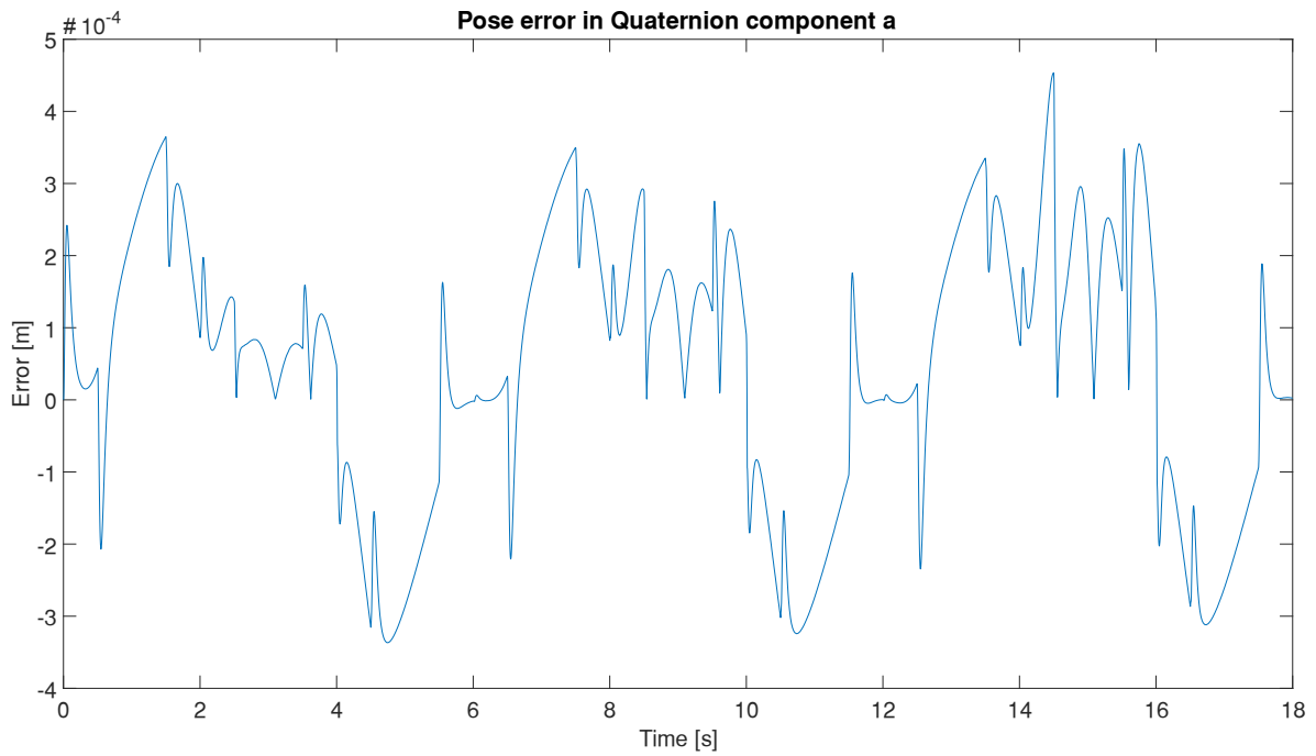
Plot 3-67. PID Controllers with Trajectory Generator. Committed error in quaternion component a .
