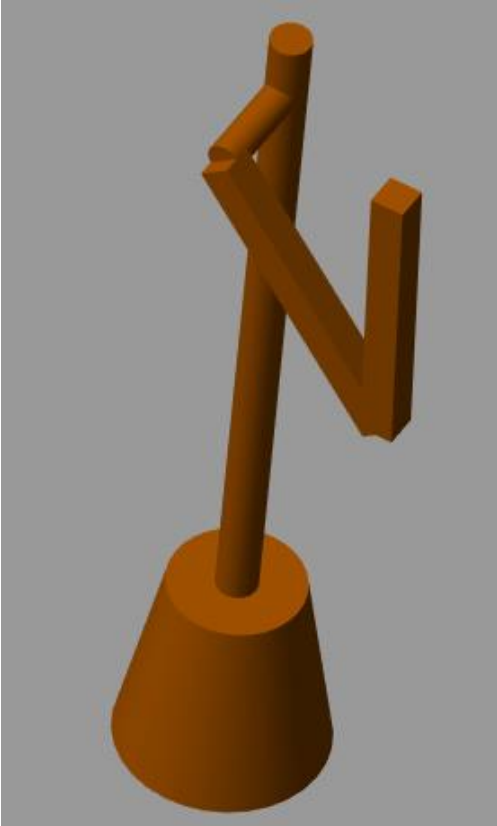
Figure 3-39. 3-D representation of the 2-link robot for testing.
