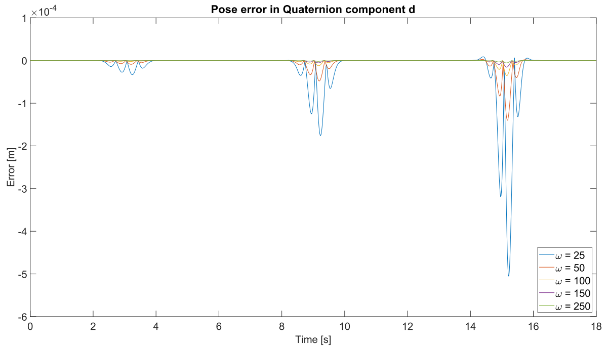
Plot 3-57. CTC Controller with Trajectory Generator. Committed error in quaternion component d .
