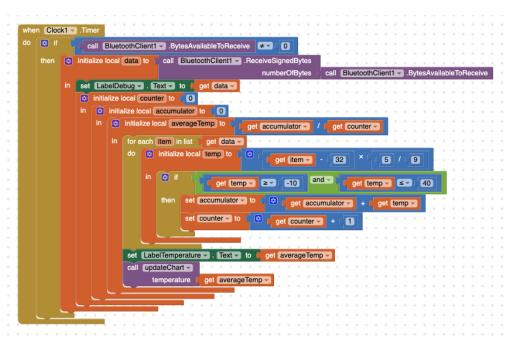
Figure 8. Processing temperature data with App Inventor.
