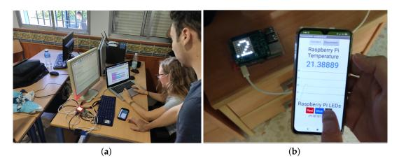
**Figure 7.** Developing the mobile app for interacting with the external Internet of Things (IoT) device. (a) Students programming the mobile app; (b) Android app communicating with the Raspberry and its Sense HAT add-on.
