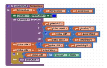
Figure 9. Drawing temperature data with App Inventor.
