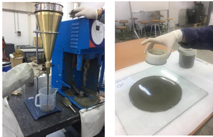
Figure 3. Marsh cone test and grout spread test for fluidity measurements.
