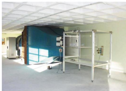
b) Test chamber of wind tunnel
