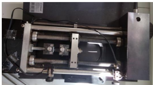
Figure 3.5: Tensile strength apparatus used to perform mechanical strength tests on PVDF and PVDF/PEDOT:PSS samples.
