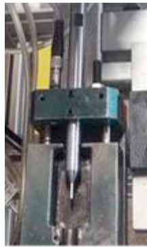
Fig. 3. Lubricant injection needle.
