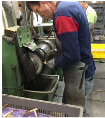
Figure 12. Manual Polishing process
