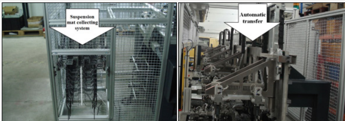
Figure 6: Applied concepts in the final station: a) Suspension mat collecting system at the final workstation; b) Automatic transfer between workstations.
