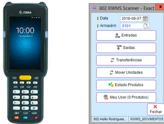
Fig. 2 – Left: Zebra MC3300 Mobile Computer, right: localization system main menu.
