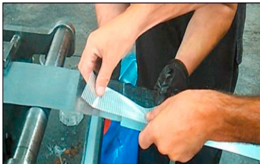
Fig. 4 – Placing the adhesive tape to join the roll plate
