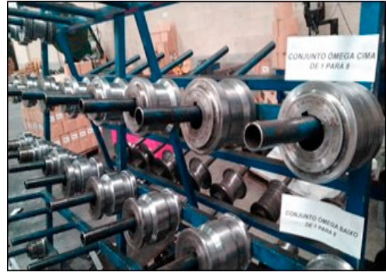
Fig. 3 – Storage of wheels of profiling machine, after 5S
