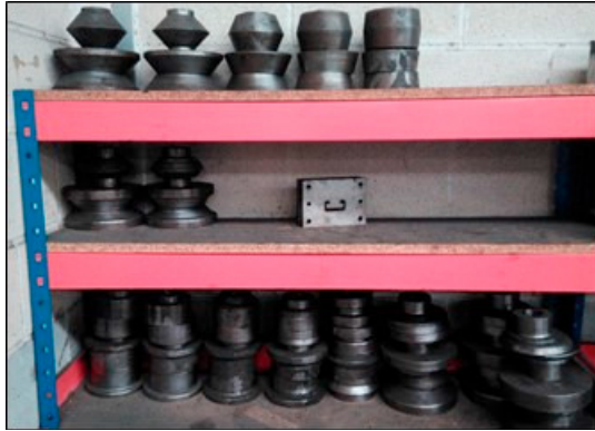
Fig. 2 – Storage of wheels of profiling machine, before 5S
