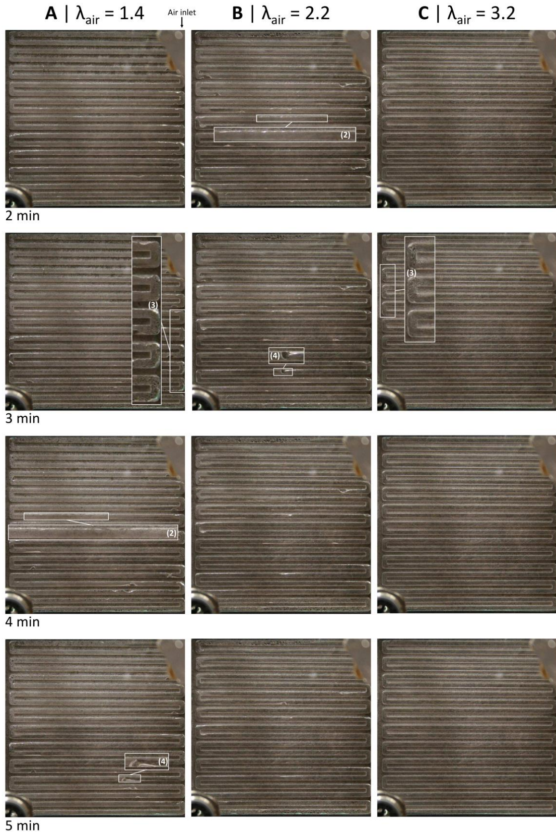
Figure 4.8. Liquid water distribution in the cathode of the transparent fuel cell over time, at 0.16 \text{ A cm}^{-2} and various air stoichiometries ( \lambda_{\text{air}} ). (1) Droplets; (2) Films; (3) Accumulation at the elbows; (4) Slugs filling most of the cross-section; (5) Slug filling the entire cross-section.
