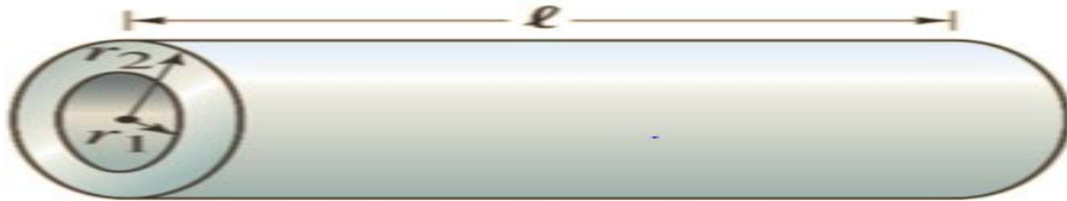
Figure 4: A hollow cylinder with length L , the internal and external radius of r_1 and r_2 respectively.
