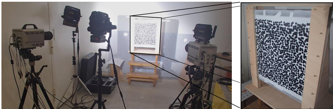
Figure 5: Stereo-correlation device comprising high speed camera and large scale target with coarse speckle pattern.
